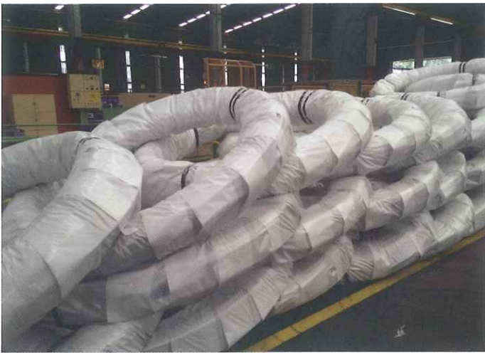
3-sided Deformed (Chevron Indented)
